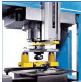
Punching tools set for diameters from 6 mm up to 40 mm with anti-deformation elastic hold-down.
