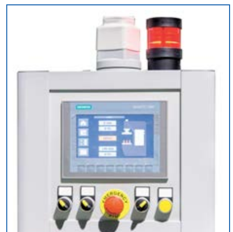
PLC SIEMENS mod. SIMATIC S7 1200 with 7" touch screen mod. KTP-700.
