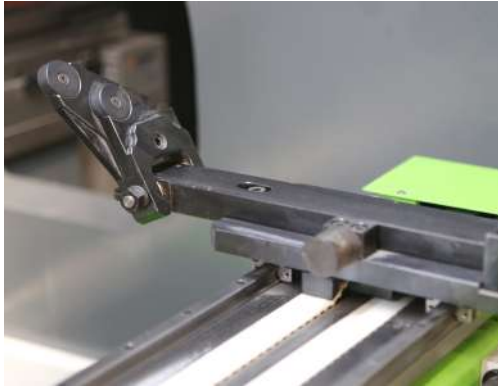
Retractable fingers which avoid collisions on "Z" reverse fold.
