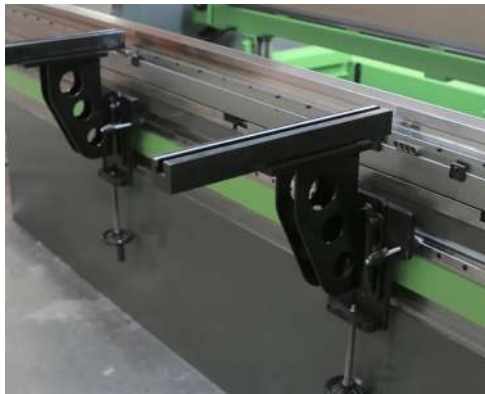
2 front supports with "T" slots with retractable millimeter stops and moveable by INA-type guides.
