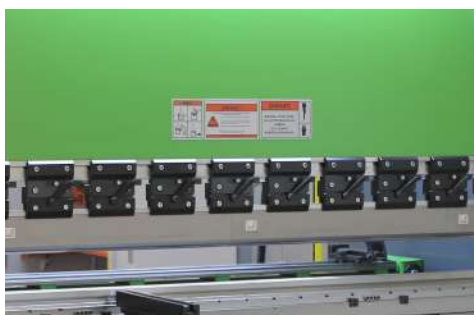
Promecam hold. Bending compensation by chocks.
